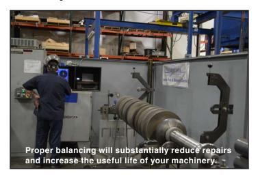
Every impeller balanced by a Tencarva Repair Center, at a minimum, conforms to a G 1.0 specification and (upon request) comes with a balance report certificate ensuring that the impeller is within the exact specifications. If even higher calibration balancing is required our equipment is capable of balance as close as a 4W/N. (4 times the weight over the service speed.)
